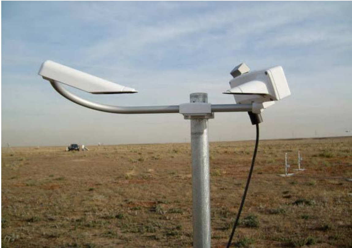
Figure 1. Vaisala PWD22 present weather detector
