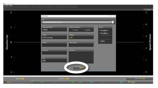
**Gomaco GSI** – After providing input for data fields in the New Datalog dialog box, select OK and press Start to begin collecting data at the Starting Station location.
