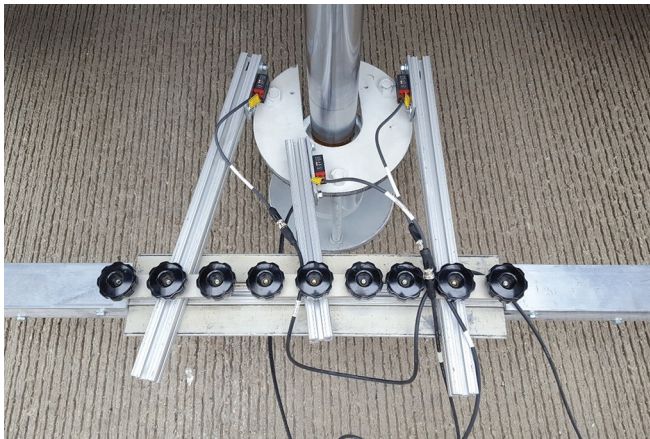
Figure 43. 12-in. diameter plate setup with reference beam for plate deflection measurements
