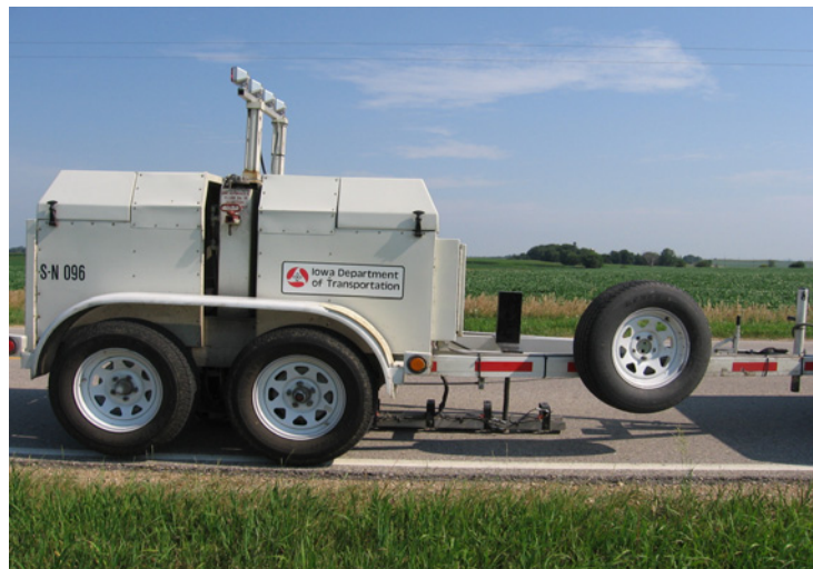
Figure 8. Picture of Iowa DOT's JILS-20 FWD equipment
