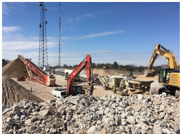
Figure 3. Crushing and sizing of source concrete at on-site stationary plant (photo courtesy of Gary Fick, Trinity Construction Management)
