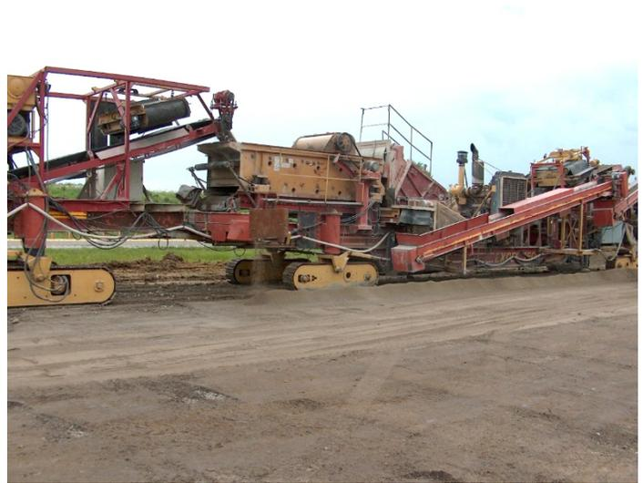
Figure 2. Mobile on-site crushing equipment (photo courtesy of Kevin Merryman, Iowa DOT)
