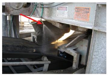
Dwayne Stenlund/MnDOT Figure 3. Spray nozzle for dust control on aggregate conveyor
