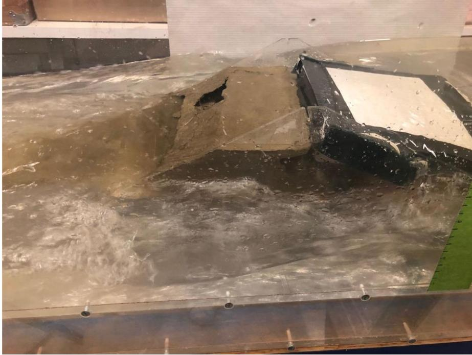
**Figure 6. No. 1 levee model during flume test**
