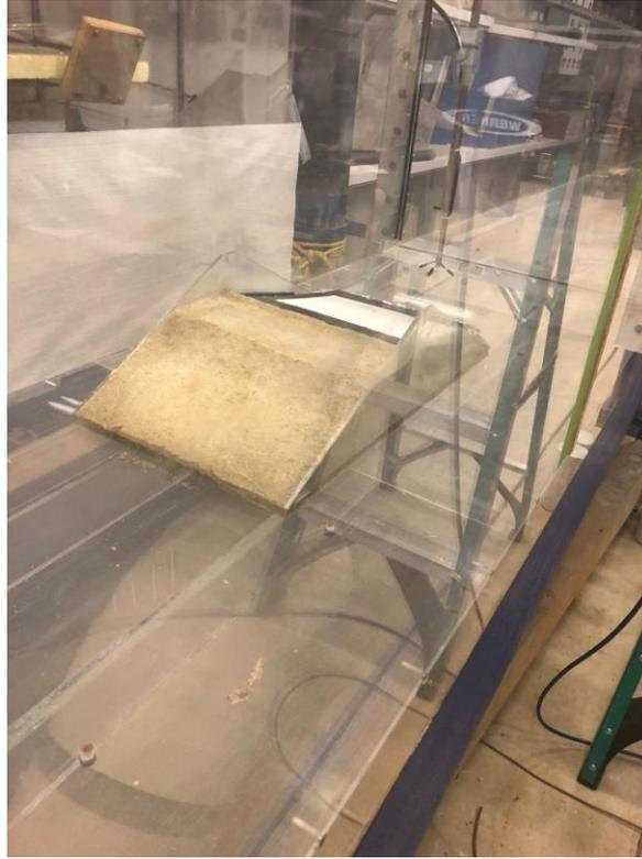
**Figure 5. No. 1 levee model flume test set up**
