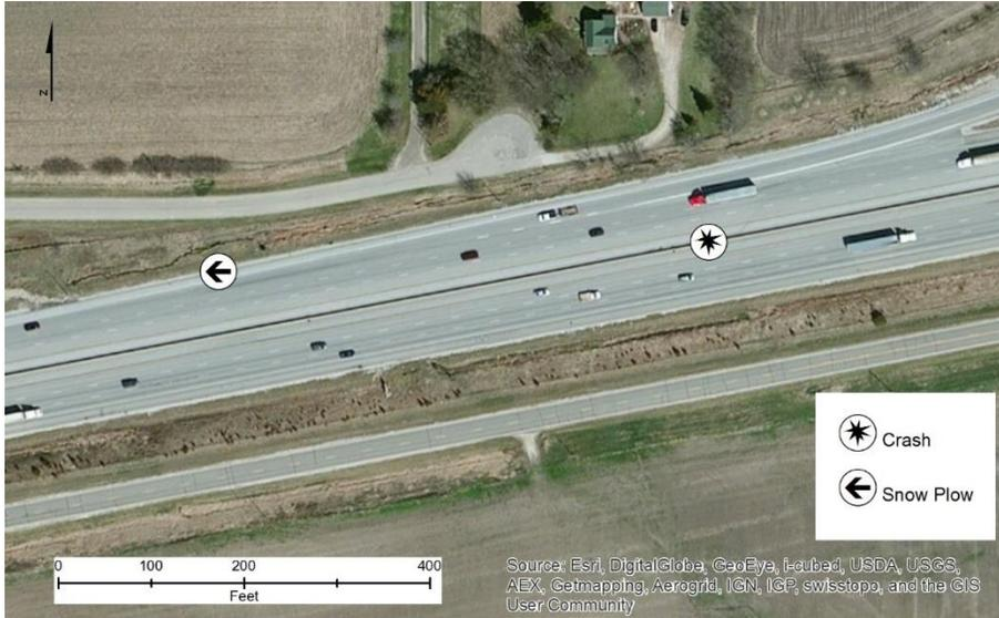
**Figure 42. Snowplow image versus crash location, Example 3**
