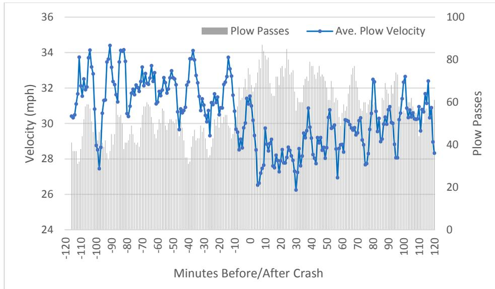
**Figure 26. Snowplow velocity and passes, 70 mph speed limit**
