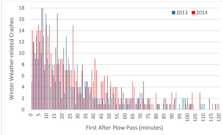
**Figure 21. First after snowplow pass, crash time interval**
