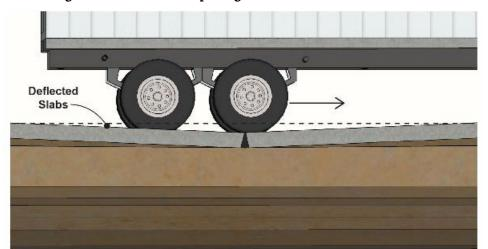
Figure 8.12 Deflection spalling mechanism without dowel bars
