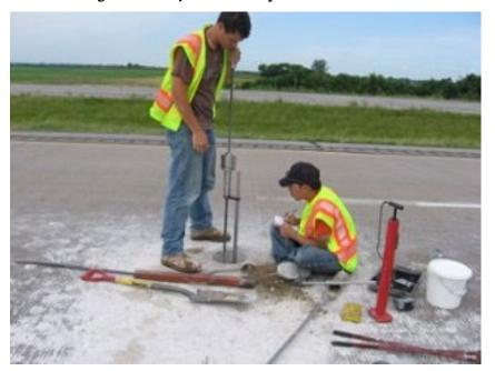
Figure 19.4 Dynamic cone penetrometer (DCP)
