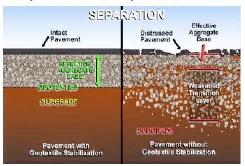
Figure 9.9 Prevention of fines into granular unstabilized subbase
