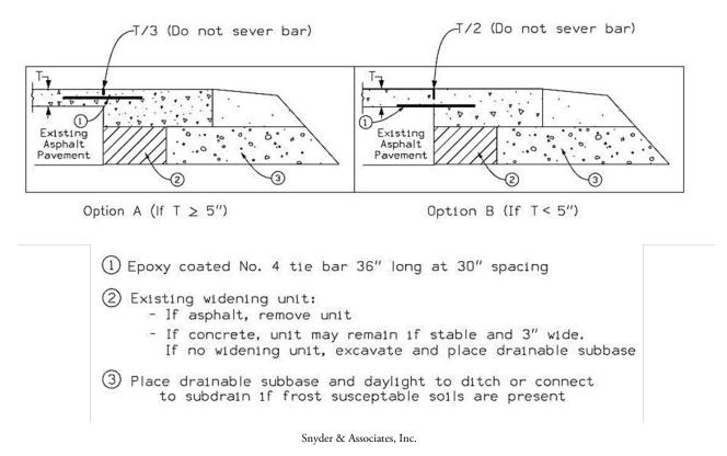
**Materials**: Tie bars should be epoxy coated with a bar size of No. 4. A 36-inch long tie bar placed at 30-inch spacing is common.
