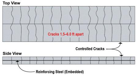
Figure 1.2 Continuously reinforced concrete pavement (CRCP)
