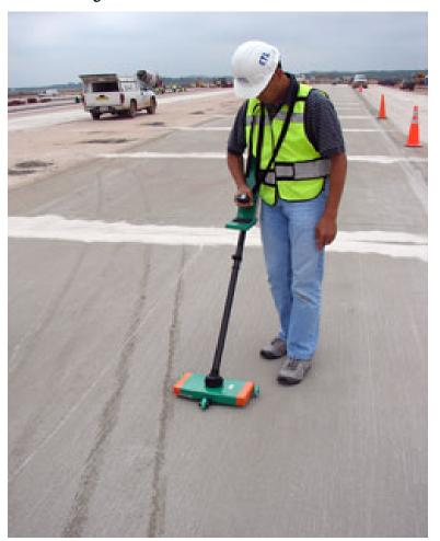
Figure 19.9 MIT-SCAN-T2 device in use
