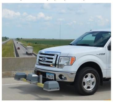
Figure 19.12 High-speed pavement profiler
