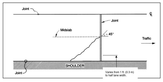
Figure 7.1 Illustration of a corner crack
