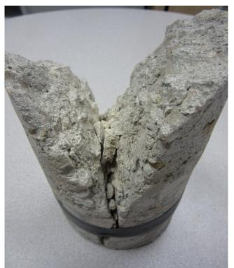
Figure 8.2 Freeze-thaw damage
