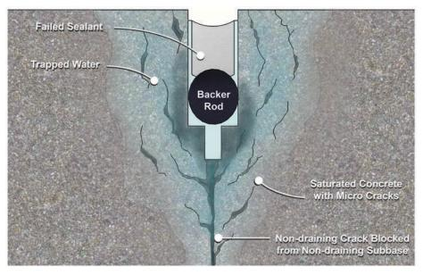
a. Poor joint sealant leading to saturation in concrete joint, resulting in micro cracking Snyder & Associates, Inc. after Jason Weiss
