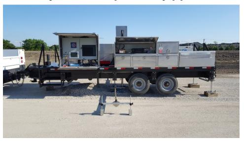
Figure 12.6 Automated plate load testing equipment
