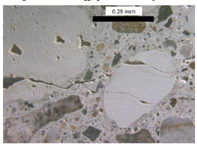
Figure 4.2 Fractured aggregate in D-cracked pavement
