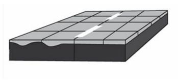
**a. Schematic of BCOA** Harrington and Fick 2014, National Concrete Pavement Technology Center
