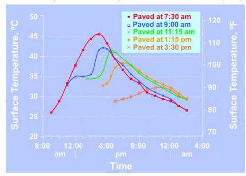
Figure 5.3 Concrete pavement surface temperatures associated with different paving times
