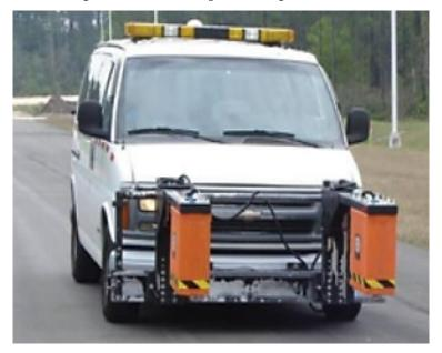
Figure 19.6 Ground penetrating radar (GPR)
