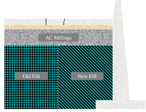
b. Cross-section of a fill section showing different fill material resulting in differential vertical movement resulting in longitudinal pavement cracking John Donahue, Missouri DOT
