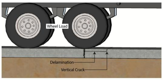
Figure 3.3 Delaminated areas leading to increased distress
