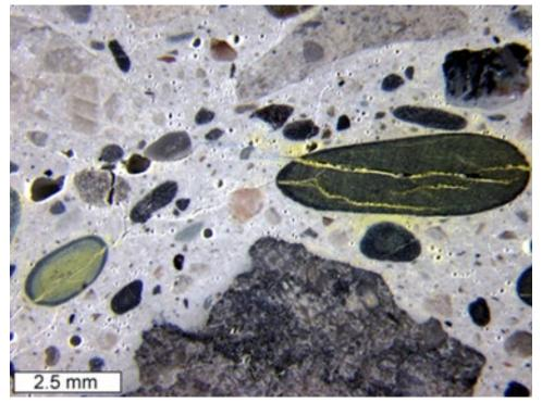
Figure 4.5 Aggregate particle fracturing due to ASR
