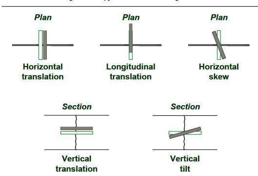
Figure 8.18 Types of dowel bar misalignment
