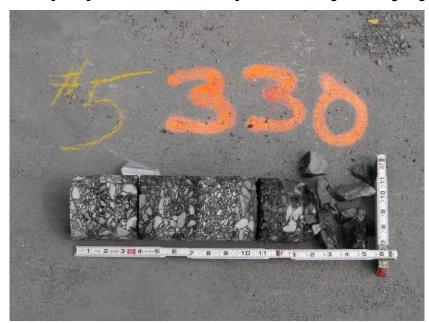
Figure 15.4 Asphalt pavement core obtained prior to selecting and designing BCOA
