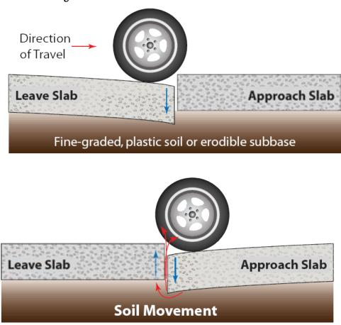
Figure 9.7 Pavement movement from eroded subbases
