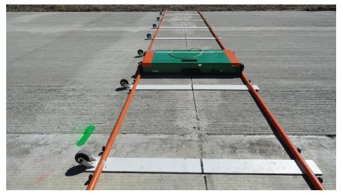
Figure 19.8 MIT Scan-2 device
