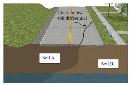
Figure 12.11 Concrete placed on natural subgrade
