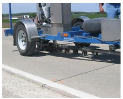
Figure 19.2 Falling Weight Deflectometer (FWD)
