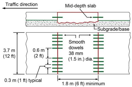
Figure 8.26 Example of full-depth repair of a spalled joint (plan view)
