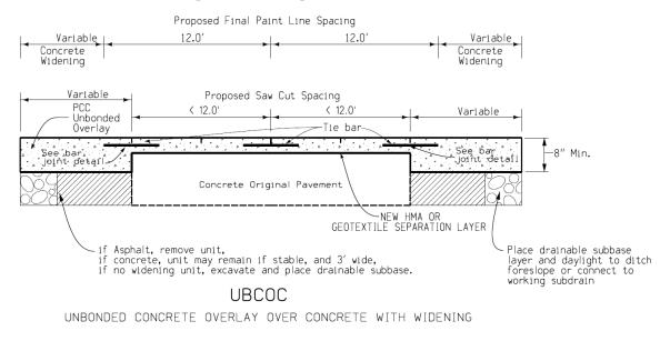
Figure 18.4 Cross-section of a proposed UBCOC design with paved widening/shoulder unit and placement of separation layer and tie bars
