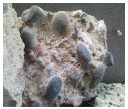
b. Loss of the damaged paste over time, leaving exposed aggregate National Concrete Pavement Technology Center
