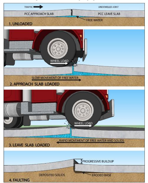
Figure 7.3 Schematic of a pumping mechanism
