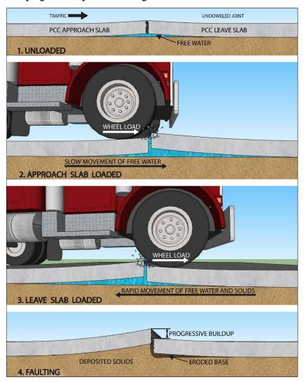
Figure 9.6 Pumping is the expulsion of subgrade soil, base, and water due to traffic loading
