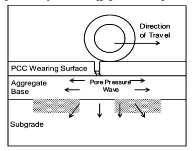
Figure 9.8 Pore pressure in the aggregate base and subgrade
