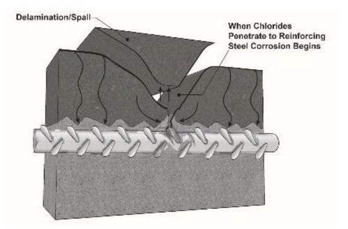
Figure 8.15 Spalling of reinforcing steel due to applications of chlorides from deicing salt
