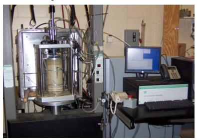
Figure 19.19 Resilient modulus test
