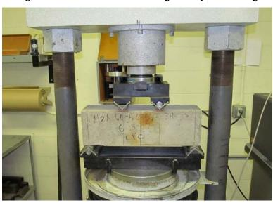
Figure 19.21 Concrete beam testing, third-point loading
