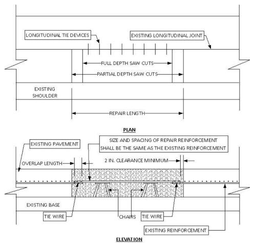
Figure 13.7 Full-depth repairs
