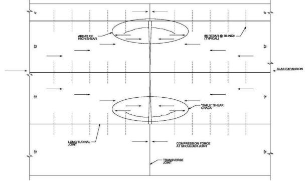
Figure 6.12 Longitudinal cracking in existing pavement with activated joints when joint movement is restrained by tying on a new adjacent lane
