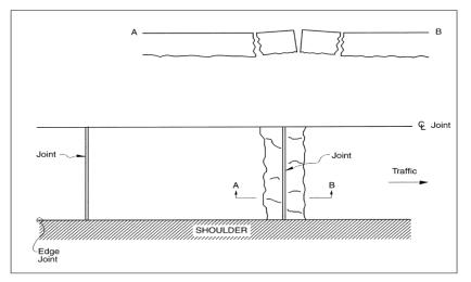
Figure 11.2 Section of Blowup in JPCP
