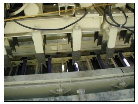
**b.** Close-up of the dowel bar inserter on a paving machine Hoegh and Khazanovich 2009, University of Minnesota
