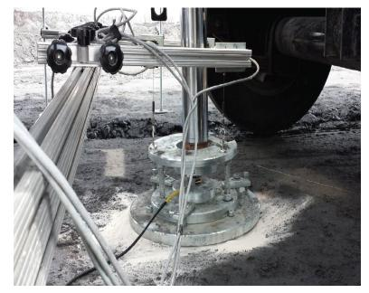
Figure 19.3 Automated plate load test
