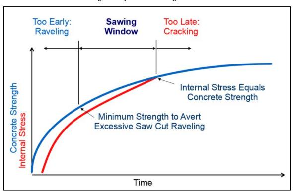
Figure 5.9 Joint saw cutting window
