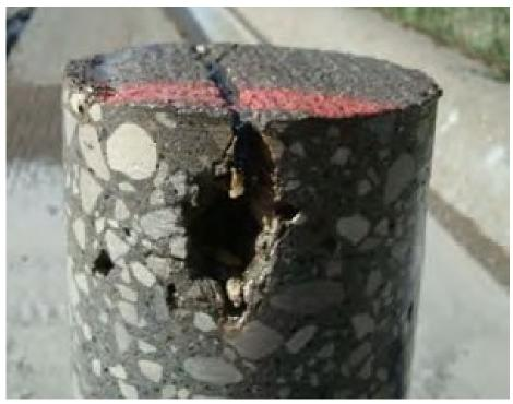
b. Longitudinal freeze damage from backer rod trapping water beneath sealant National Concrete Pavement Technology Center
