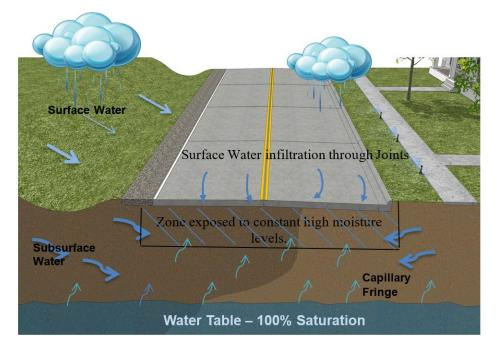
Figure 12.3 Concrete pavement exposed to surface and subsurface moisture conditions
