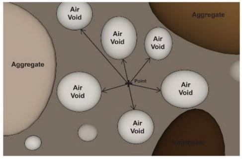
Figure 8.6 Spacing factor is the average distance from any point to the nearest air void
