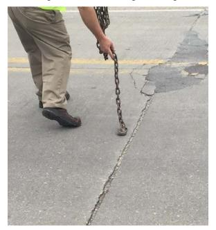
Figure 19.1 Chain drag sounding
