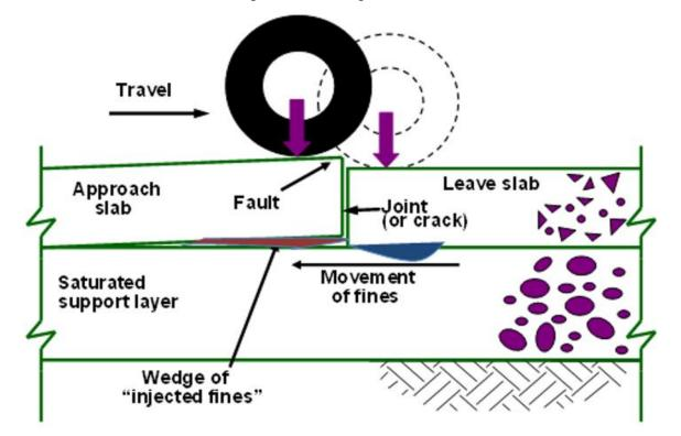
Figure 9.2 Faulting mechanism
