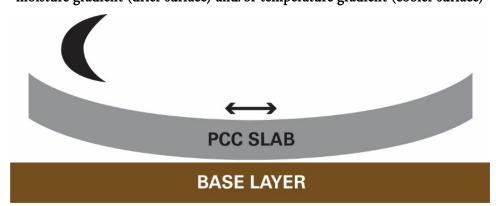
Figure 7.7 Schematic showing upward curl and loss of support near slab corners in response to moisture gradient (drier surface) and/or temperature gradient (cooler surface)
