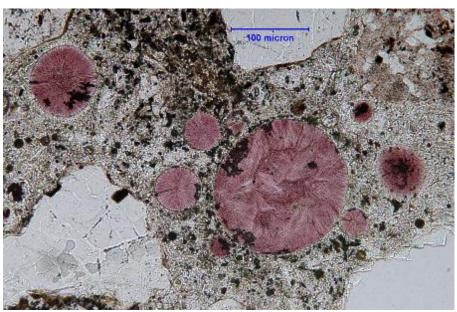
Figure 8.8 Secondary ettringite crystals in air voids
