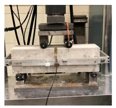
Figure 6. ASTM C1609 beam test for FRC materials
