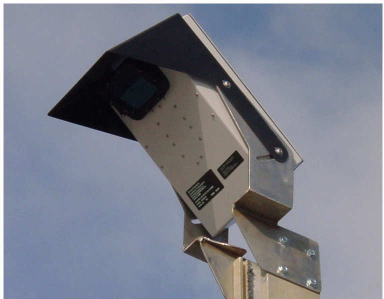
LRSS sensor module and mounting bracket
