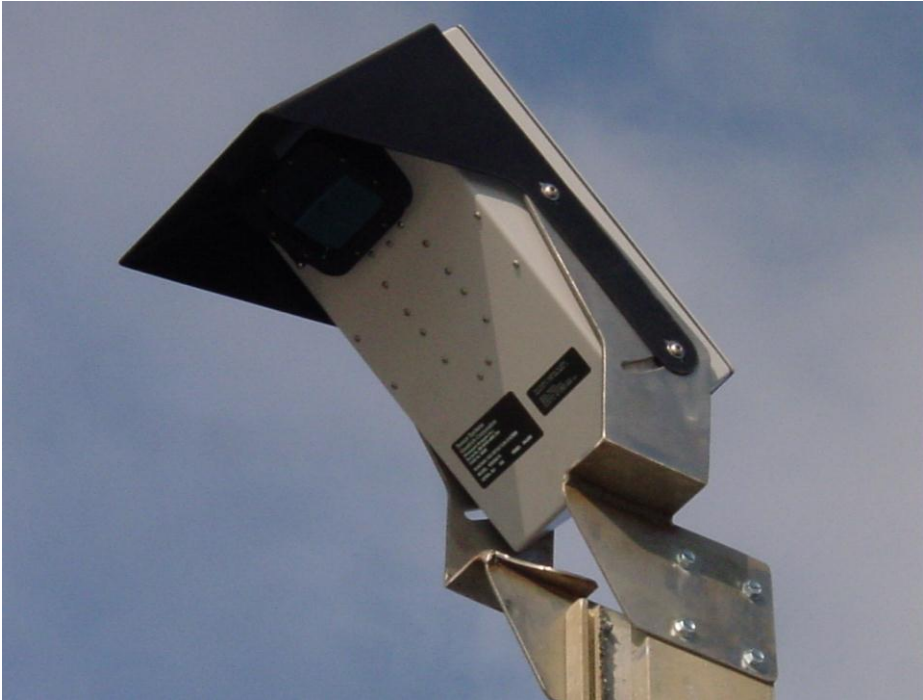
Figure 2. LRSS sensor module and mounting bracket
