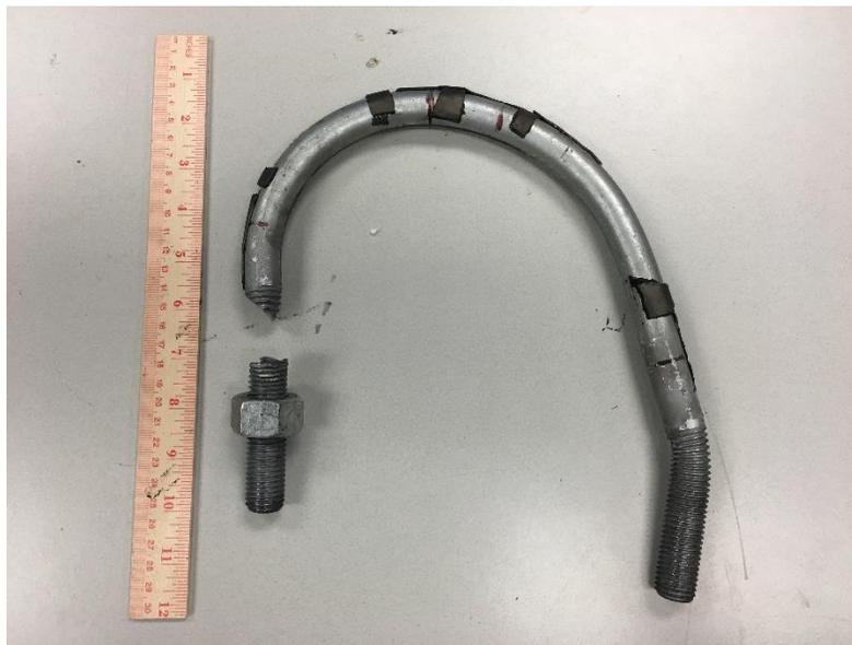
**Figure 28. Shear failure on the U-bolt shanks (Type-B, horizontal loading)**
