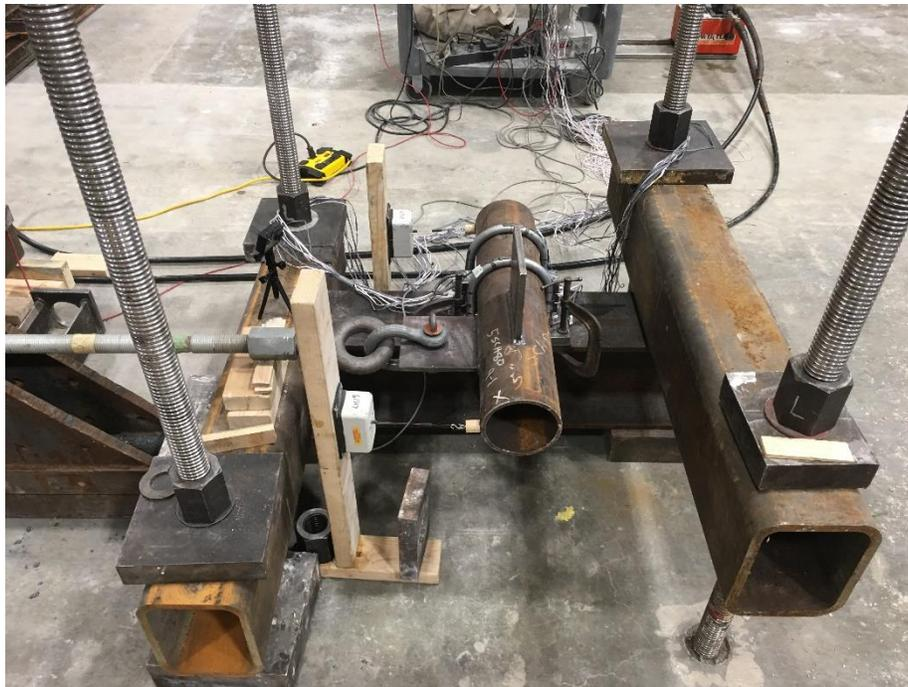
(a) Type-A specimen subjected to horizontal load
