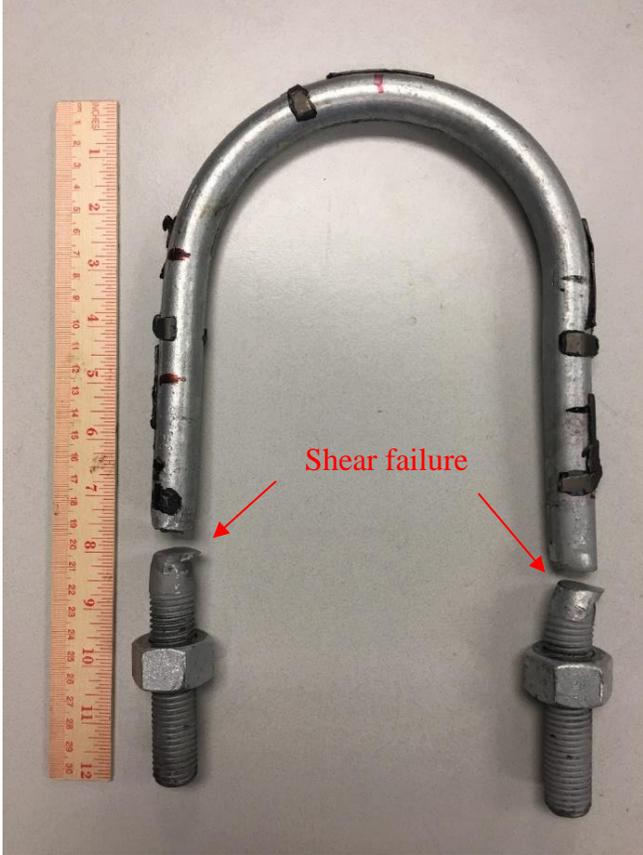
**Figure 13. Shear failure on the U-bolt shanks (Type-A, horizontal loading)**
