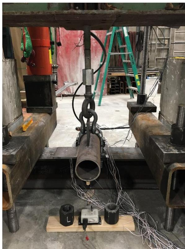
(b) Type-A specimen subjected to vertical load
