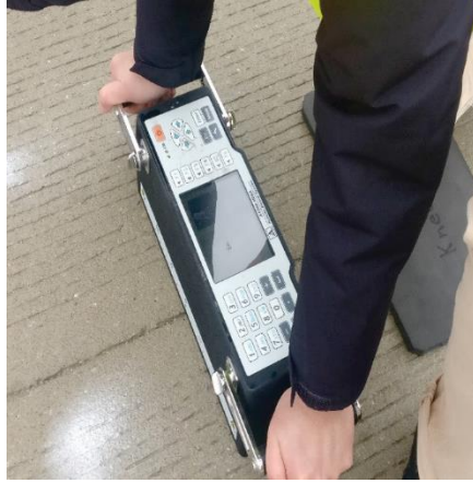
Figure 3. MIRA device used to gather joint activation data
