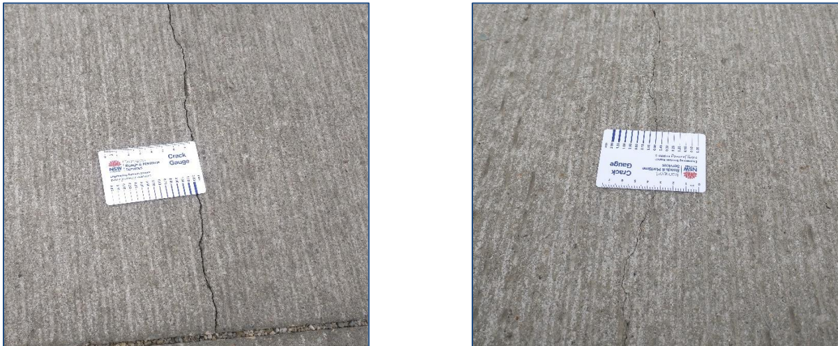
Figure 47. Comparison of reflective cracks developed in test sections without fibers (left) to those with fiber reinforcement (right)
