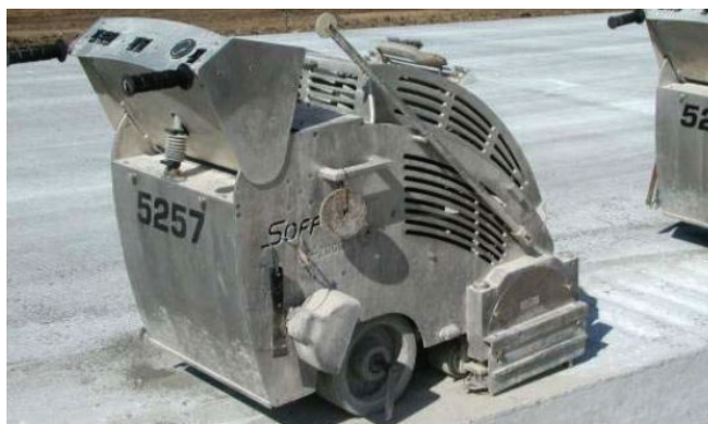
Figure 39. Early-entry concrete saw
