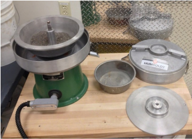
Figure 4. Illustration of the centrifuge, which has been used to determine the moisture properties of fine LWA
