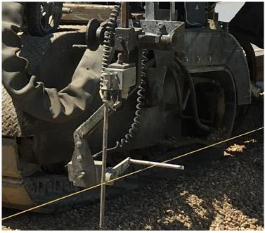
The Transtec Group, Inc. Figure 15. Paver sensor in contact with the stringline
