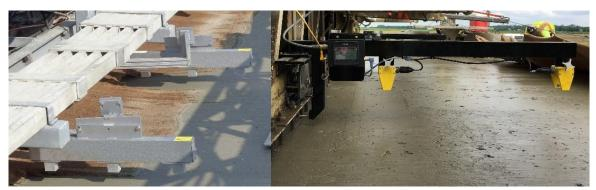
Ames Engineering (left) and GOMACO (right) Figure 26. RTS devices installed on slipform pavers
