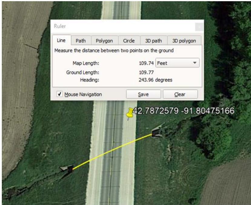
**Figure 20. Length of culvert measured manually in Google Earth**
