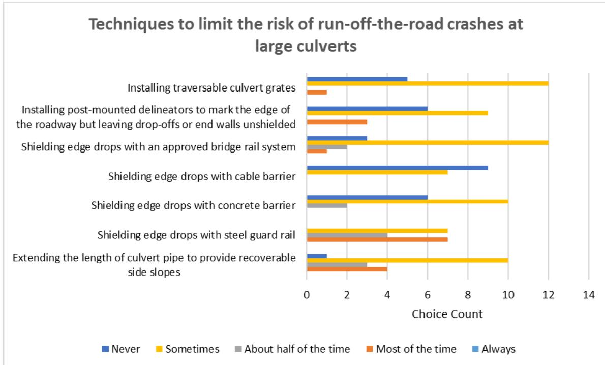
**Figure 3. Selection of techniques to limit the risk of run-off-road crashes at large culverts**
