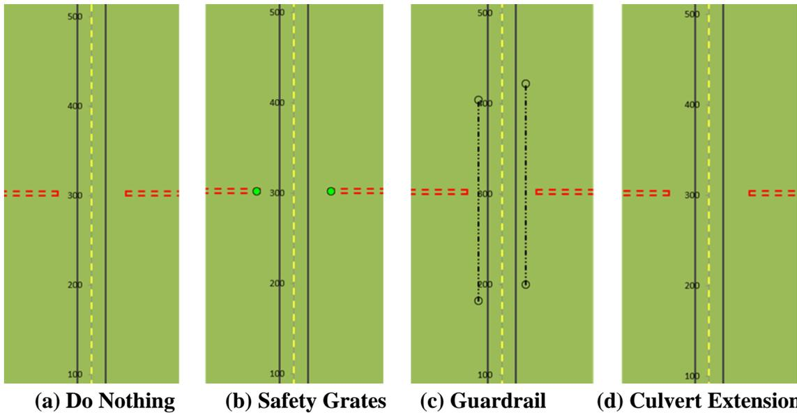
**Figure 24. RSAP alternatives for medium pipe culvert on two-lane 55 mph undivided highway**
