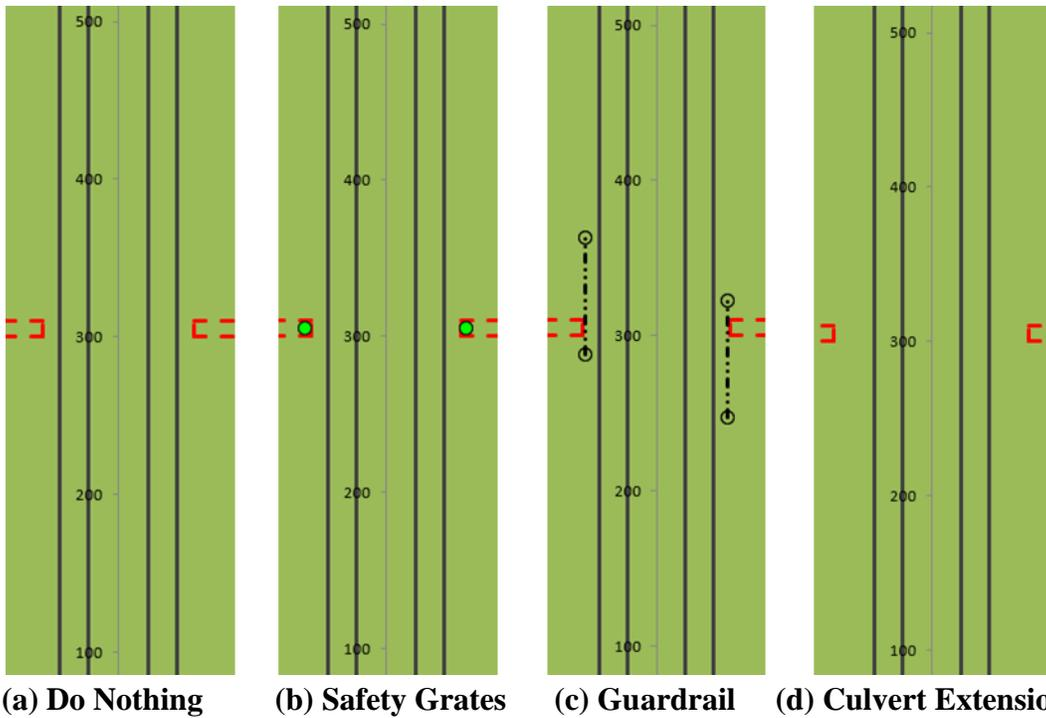
**Figure 25. RSAP alternatives for large box culvert on four-lane 70 mph divided highways**
