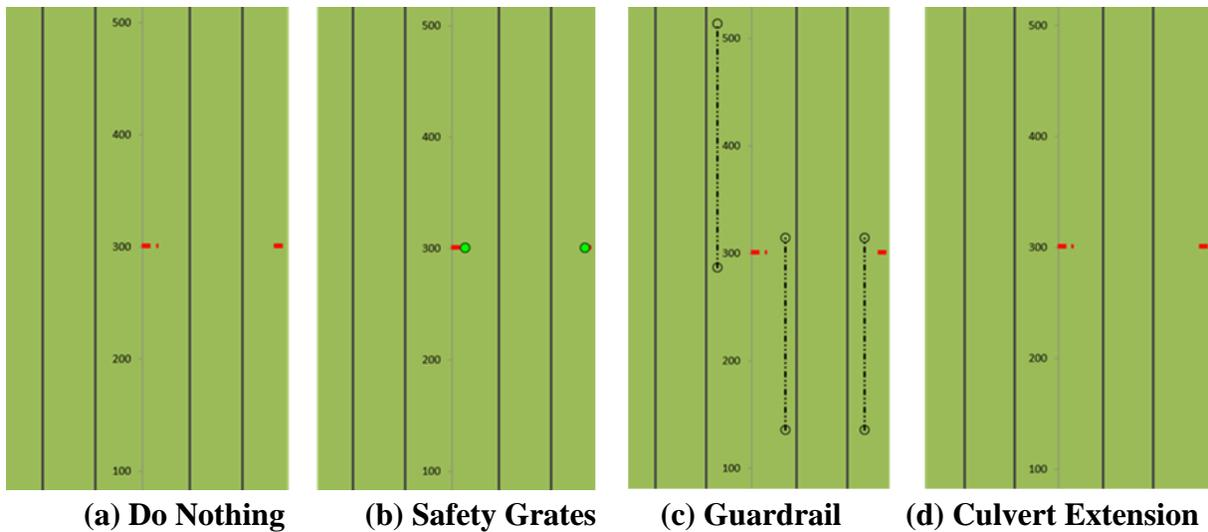
**Figure 26. RSAP alternatives for a small pipe median culvert on four-lane 70 mph divided highways**
