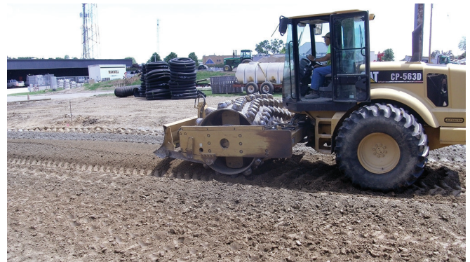
Figure 5.7. Vibratory sheepsfoot tamping roller
