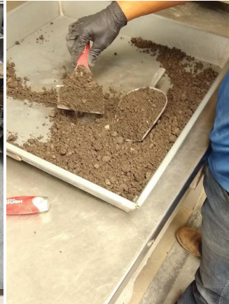
Figure B.2. Mixing additive and soil in the laboratory
