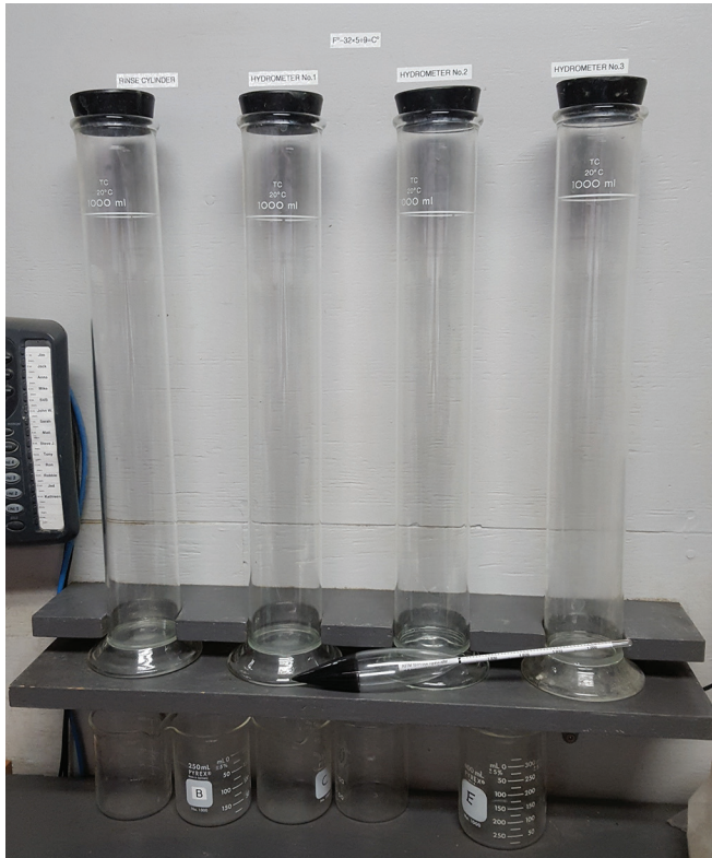
Figure 2.5. Hydrometer test apparatus
