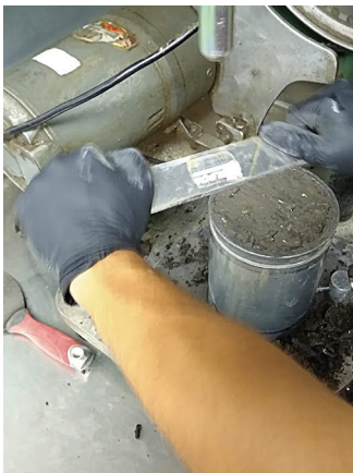
Figure B.3. Preparing a specimen just after compaction
