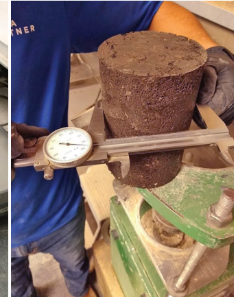
Figure B.6. Measuring the diameter of a specimen
