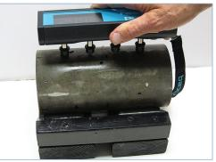
Cylinder sample testing with surface resistivity meter
