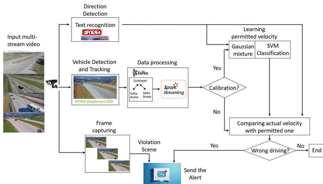
*Flow of the fully automated wrong-way driving detection system when DeepStream produces detection and tracking results*
