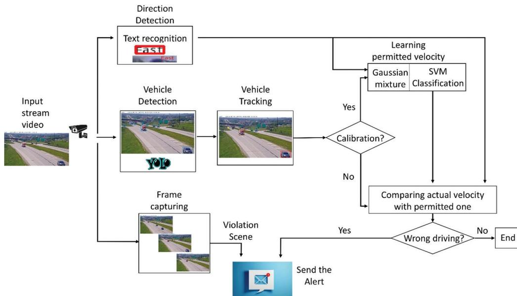
*Flow of the fully automated wrong-way driving detection system when YOLOv3 acts as the detector with SORT as the tracker*
