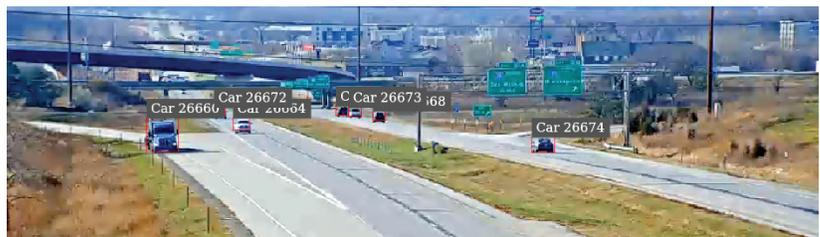
Sample output from DeepStream model where DeepStream does both vehicle detection and tracking
