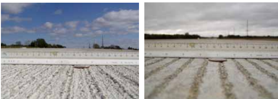
Figure 3. Two longitudinally-tined concrete pavements with average OBSI tire-pavement noise levels of 99 dBA (left) and 105 dBA (right)
