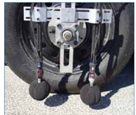
Figure 1. On-board sound intensity (OBSI) test method with view of microphones mounted in close proximity to the tire contact patch
