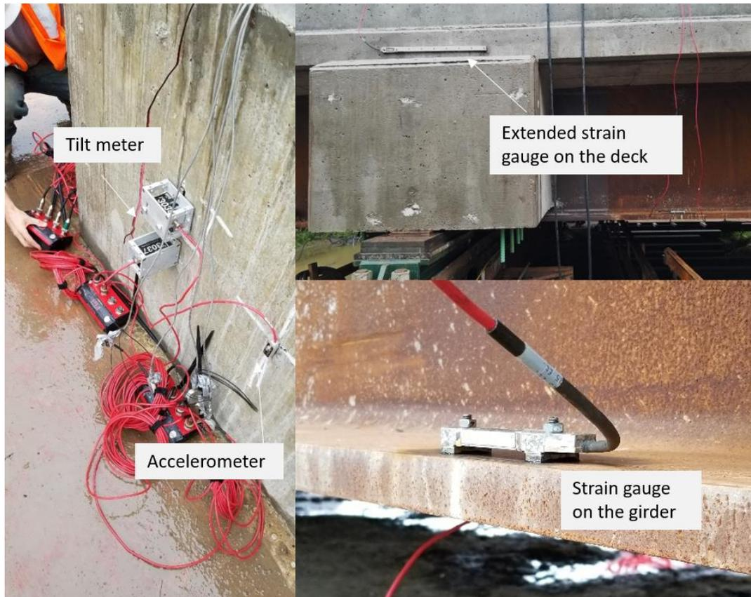
**Figure 9. Instrumentation**
