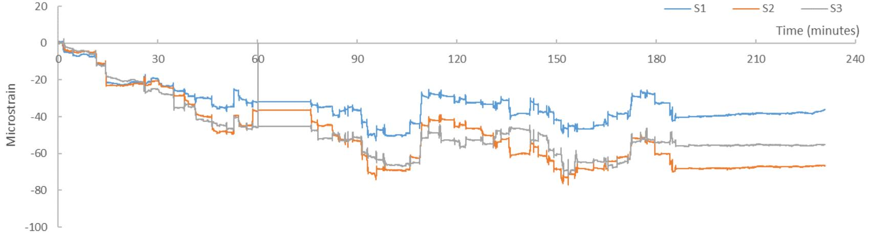
**Figure 28. Girder strain data from S1, S2, and S3**
