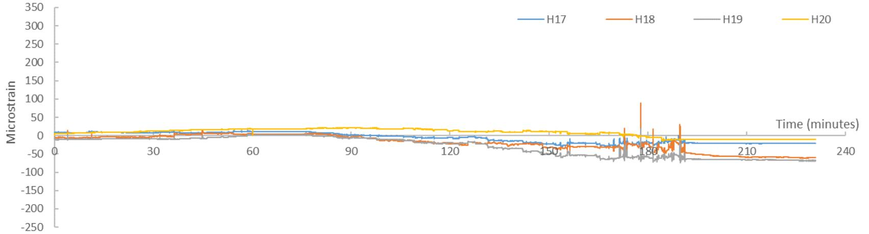
**Figure 25. Pile strain data from H17, H18, H19, and H20**
