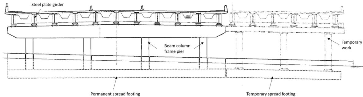
a) Beam-column frame pier on spread footing (I-405 over NE 8th Street, Washington)
