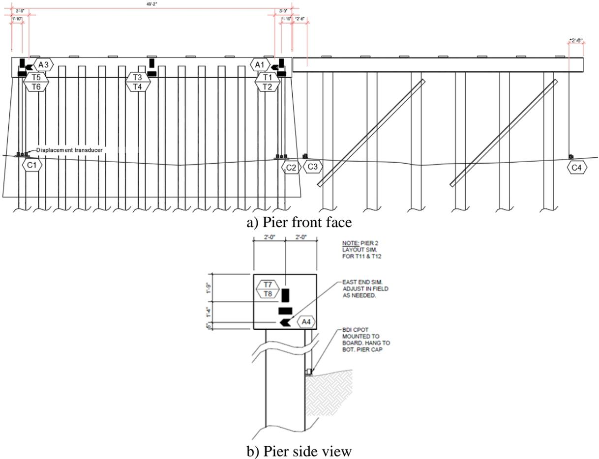
**Figure 11. Pier 1 instrumentation**
