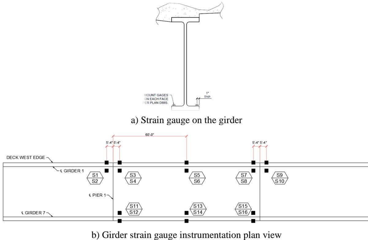
**Figure 13. Strain gauges installed on the girders**
