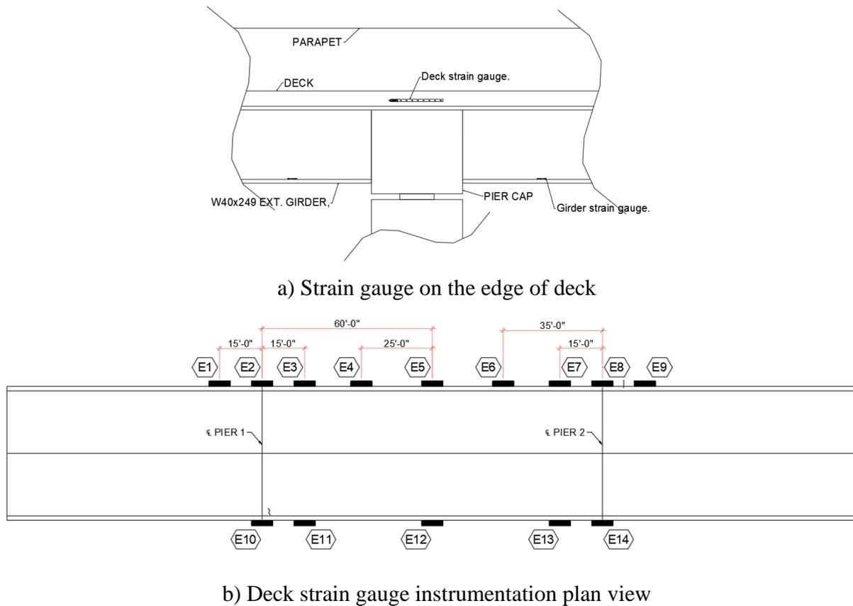
**Figure 12. Extended strain gauges installed on the deck**
