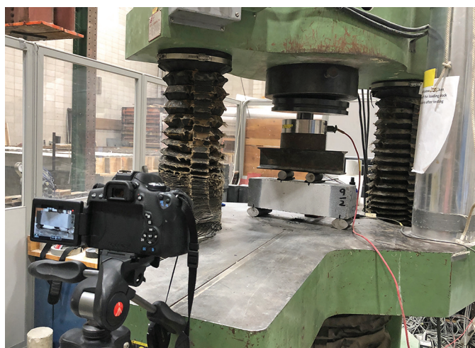
Test setup used to capture flexural response of developed non-proprietary UHPC mixtures in the laboratory
