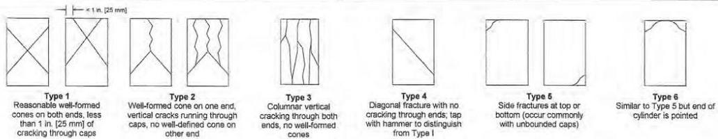
ASTM C39 Compressive Strength of Concrete Cylinders
