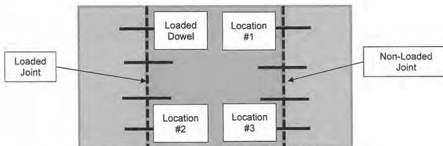
Figure 11. Secondary Deflection Measurement Locations
