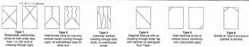
**ASTM C39 Compressive Strength of Concrete Cylinders
