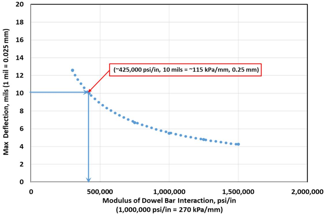
**Figure 5. Plot of 2016 FE analysis of AASHTO T 253 load-deflection test for various values of K**
