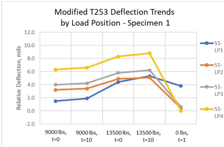
**Figure 9. Plot of relative deflection data for each load position of modified AASHTO T 253 load-deflection test Specimen 1 at each stage of test protocol (t = 0 minutes)**
