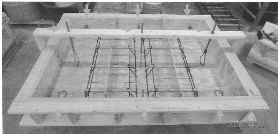
**Figure 5. Modified Sample Forms (Red Arrows Indicating the Drop-In Anchors)**
