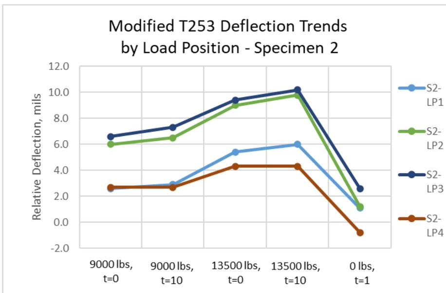
**Figure 10. Plot of relative deflection data for each load position of modified AASHTO T 253 load-deflection test Specimen 2 at each stage of test protocol (t = 0 minutes)**
