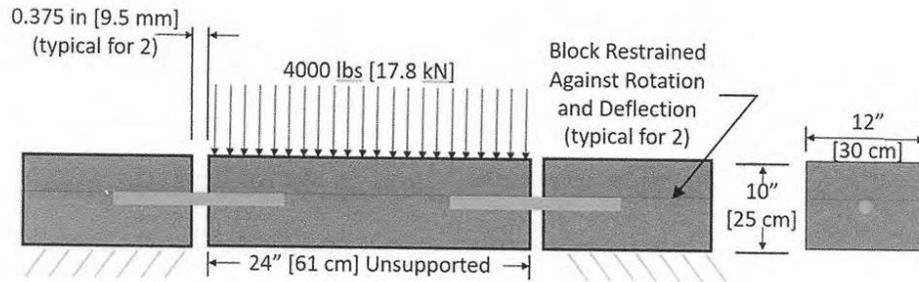
Figure 1. Standard AASHTO T253 Specimen and Test (As Provided by ACPA)
