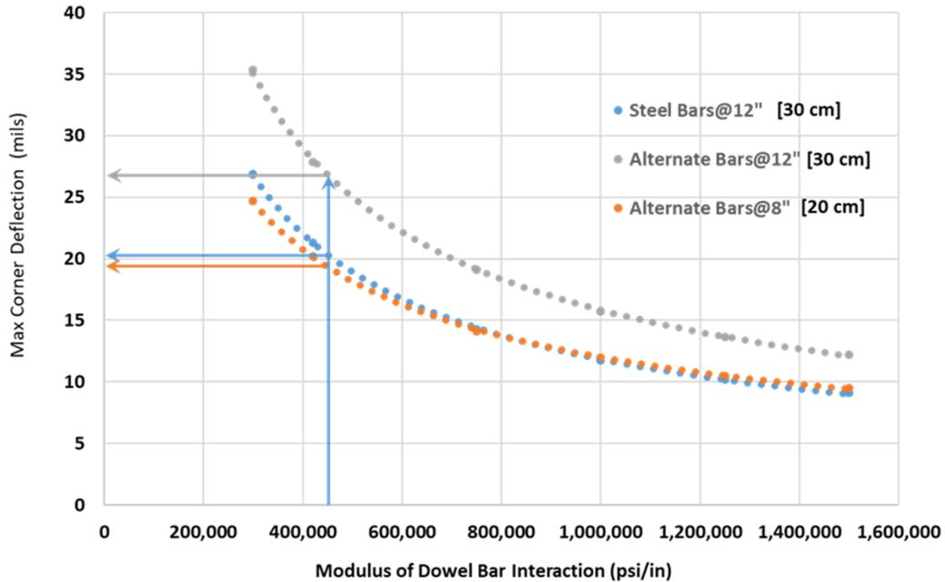
**Figure 6. Plot of 2016 FE analysis results for modified AASHTO T 253 load-deflection test for various values of K and various dowel types and spacing**
