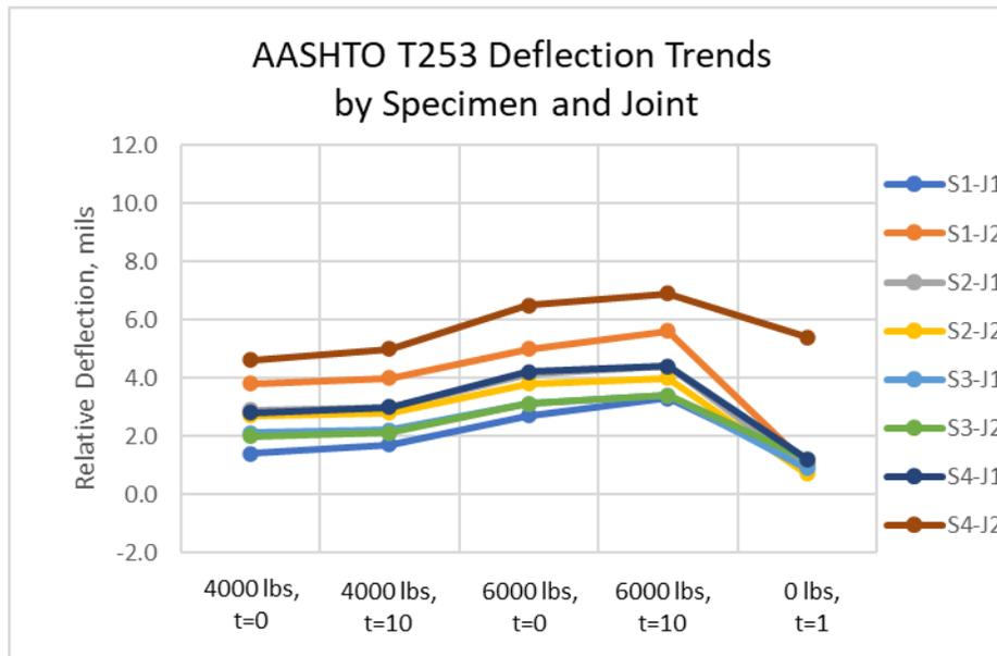
**Figure 7. Plot of relative deflection data for each joint of AASHTO T 253 load-deflection test specimen at each stage of test (t = 0 minutes)**
