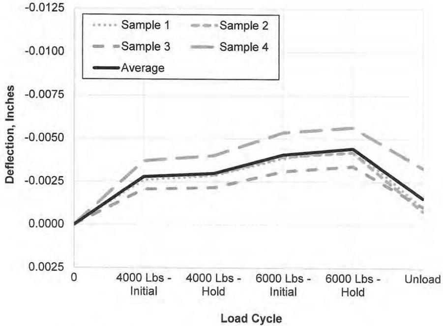
Figure 10. Load and Deflection History for the Standard Sample Test
