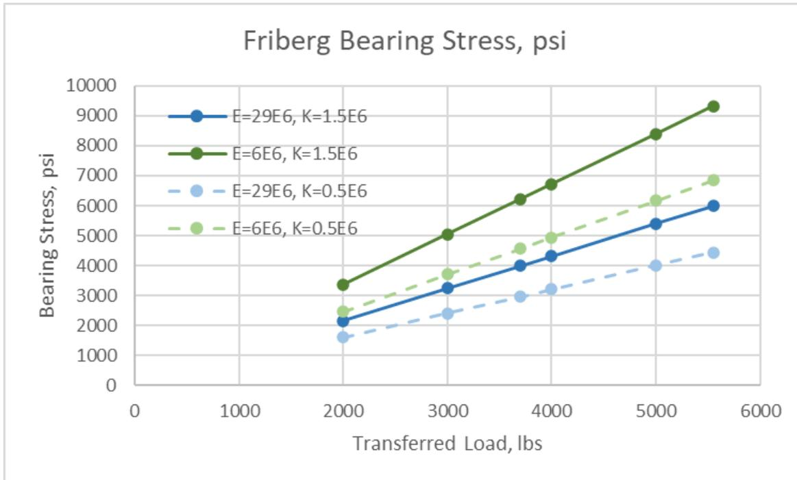
**Figure 12. Calculated bearing stresses for critical dowel in modified AASHTO T 253 load-deflection test for a range of transferred shear loads and selected dowel modulus and K values**
