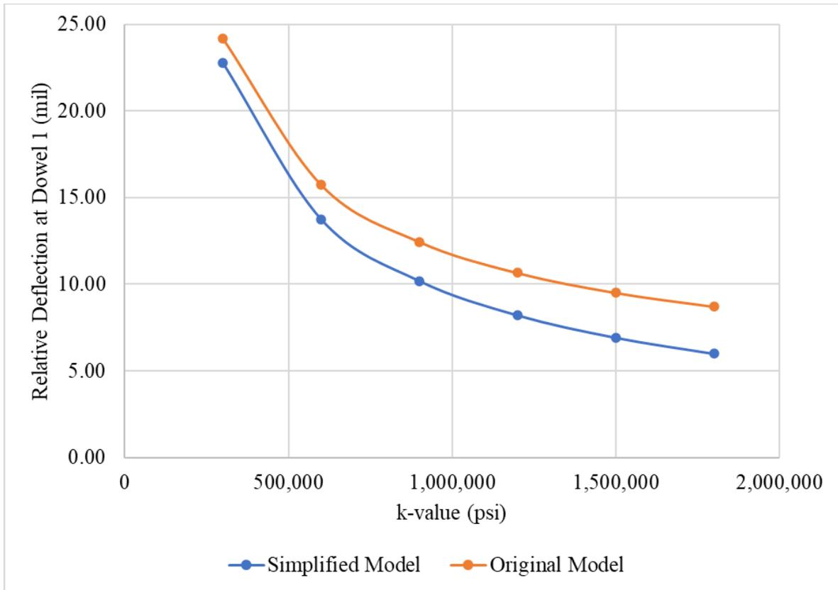
**Figure 15. Graph of relative deflection versus K for the modified AASHTO T 253 load-deflection test for the original and updated finite element models (data for Dowel Bar 1 only [under the applied load] from Table 6)**
