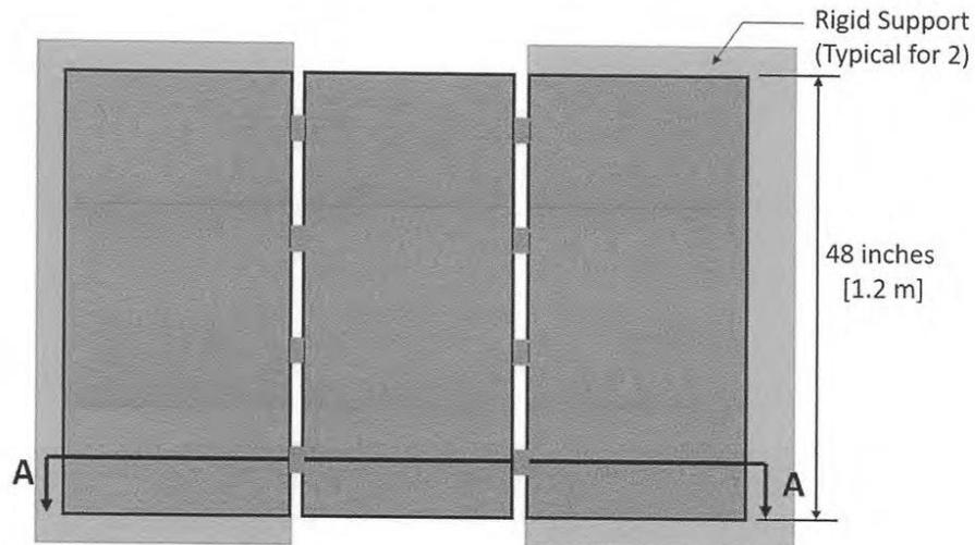
Figure 2. Modified Test Specimen – Plan View (As Provided by ACPA)
