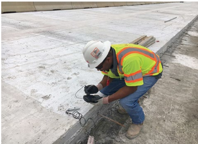
Figure 5.14. Maturity testing of concrete pavement
