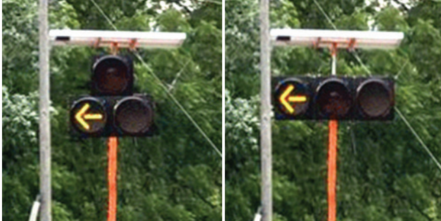
Recommended DAD signal head configuration alternatives (doghouse and horizontal)
