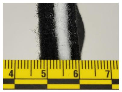
Figure 1. Edge view of the three geotextile samples evaluated
