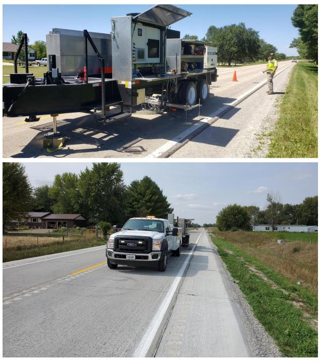
Figure 15. APLT equipment setup on the existing ACC layer (top) and after PCC overlay (bottom)
