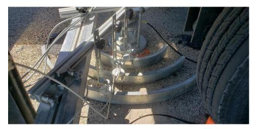
Figure 17. 12 in. diameter plate setup with reference beam for deflection basin measurements on ACC pavement prior to constructing the overlay
