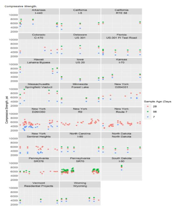
Figure 60. Compressive strength for various locations
