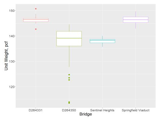
Figure 38. Unit weight box and whisker data for bridges
