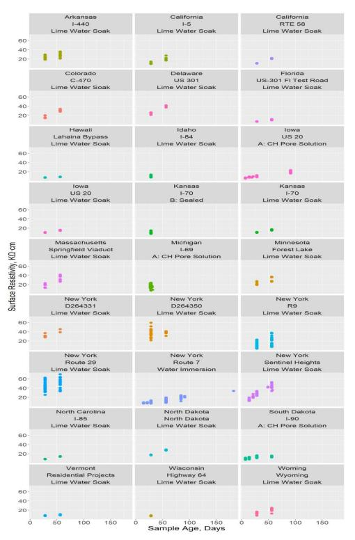
Figure 68. Surface resistivity versus age for various locations
