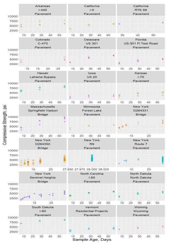
Figure 63. Compressive strength data for pavements at various locations
