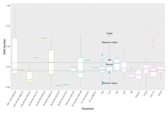
Figure 39. SAM box and whisker data for pavements
