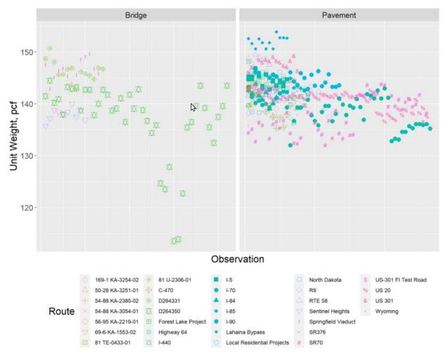
Figure 35. Unit weight scatter data for bridges and pavements
