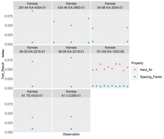
Figure 56. Hardened air and spacing factor
