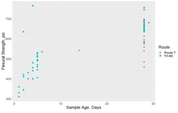
Figure 64. Flexural strength data for pavements
