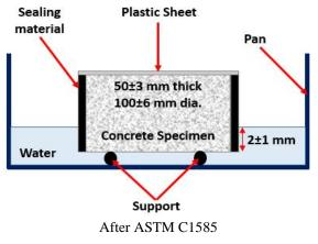
Figure 4. Specimen setup in ASTM C1585
