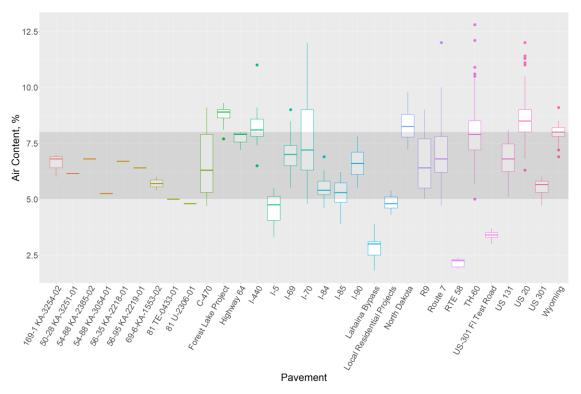
Figure 45. Air content box and whisker for pavements
