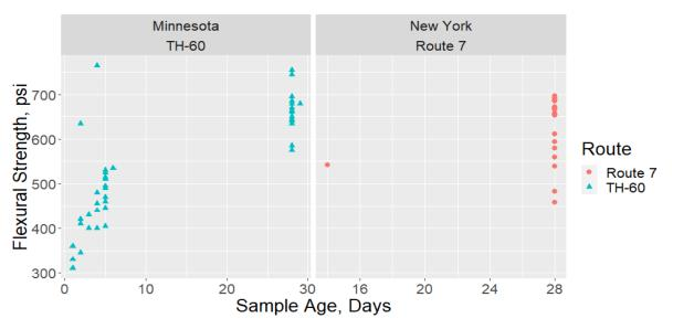
Figure 65. Flexural strength data for pavements at various locations
