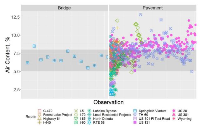
Figure 47. Air content scatter data for bridges (left) and pavements (right)
