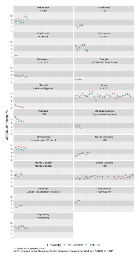
Figure 48. Air content measured by Type B meter (Air\_Content) and SAM (SAM\_Air) for various locations
