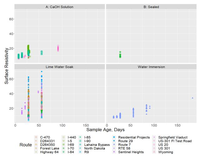
**Figure 17. Surface resistivity for various preparation conditions**
