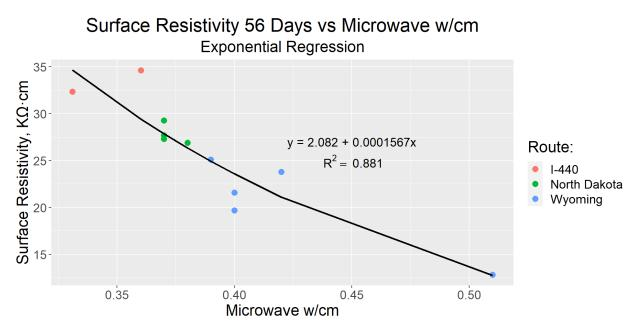
Figure 73. Surface resistivity versus microwave w/cm ratio
