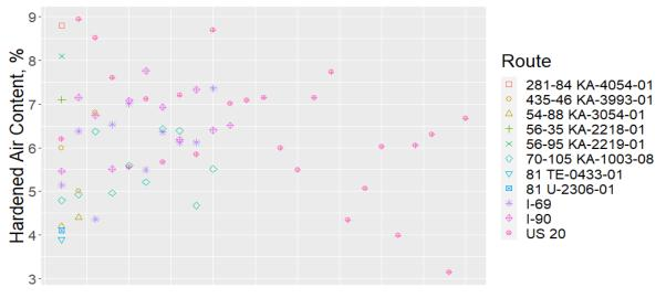
Figure 57. Scatter data for hardened air content
