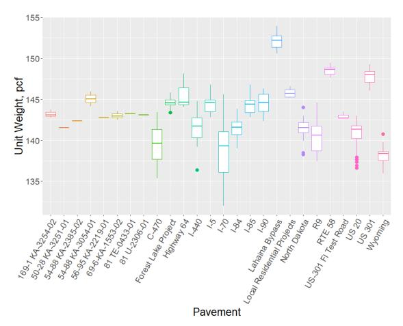
Figure 37. Unit weight box and whisker data for pavements
