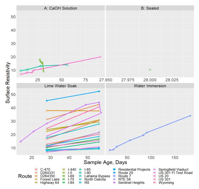
Figure 18. Surface resistivity versus age for various preparation conditions
