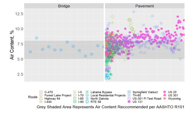
Figure 16. Air content for bridge and pavement projects
