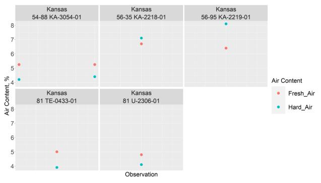
Figure 51. Fresh and hardened air content
