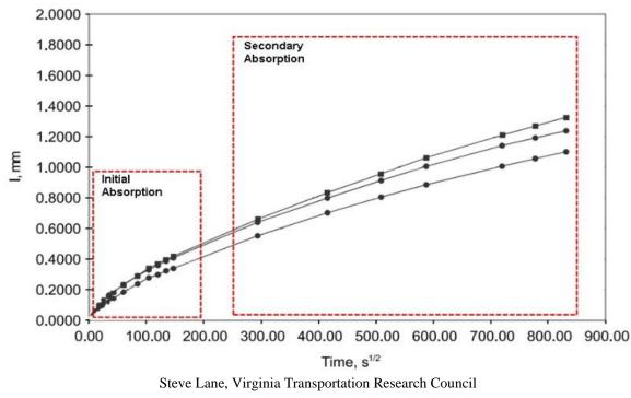
Figure 5. Initial and secondary absorption
