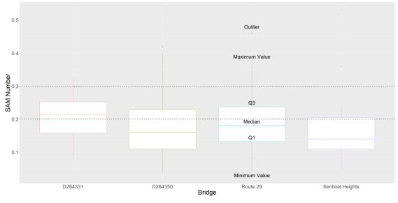
Figure 40. SAM box and whisker data for bridges
