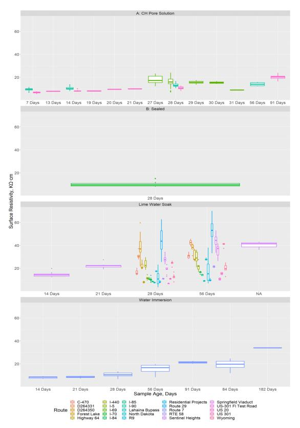
Figure 70. Box and whisker data for surface resistivity versus age for various conditioning methods
