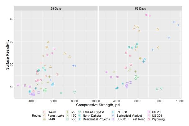
Figure 66. Scatter data for surface resistivity versus compressive strength
