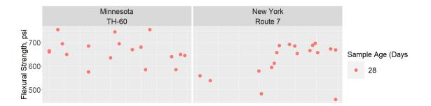
Figure 61. Flexural strength for various locations
