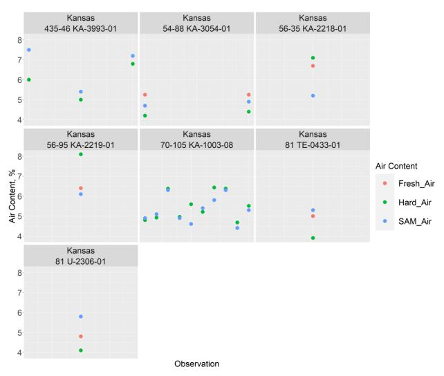
Figure 53. Fresh air, hardened air, and SAM air
