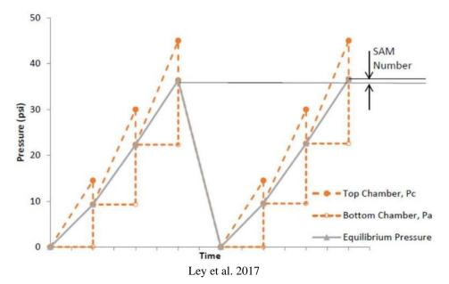
Figure 8. Sequential pressures applied in the SAM and calculation of the SAM number
