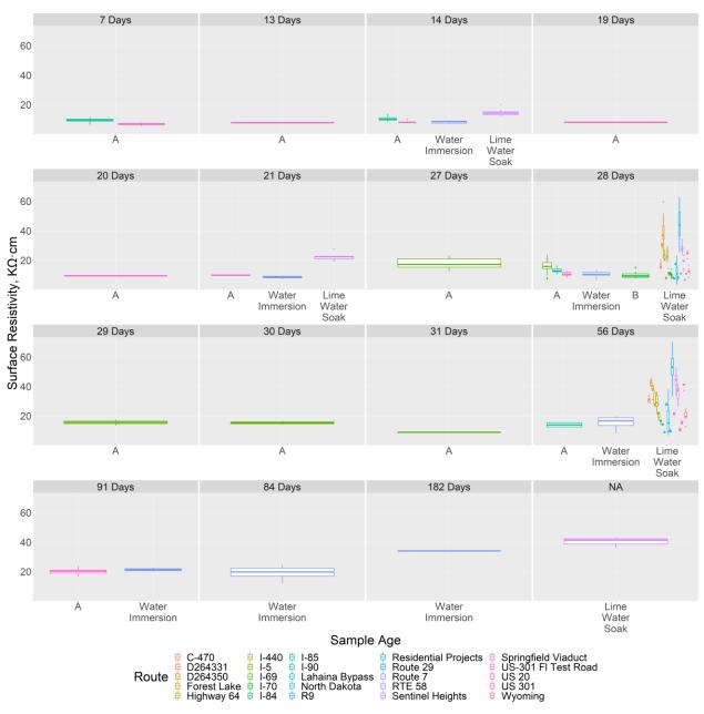
Figure 71 shows box and whisker plots for the resistivity of samples conditioned by various methods for various projects.
