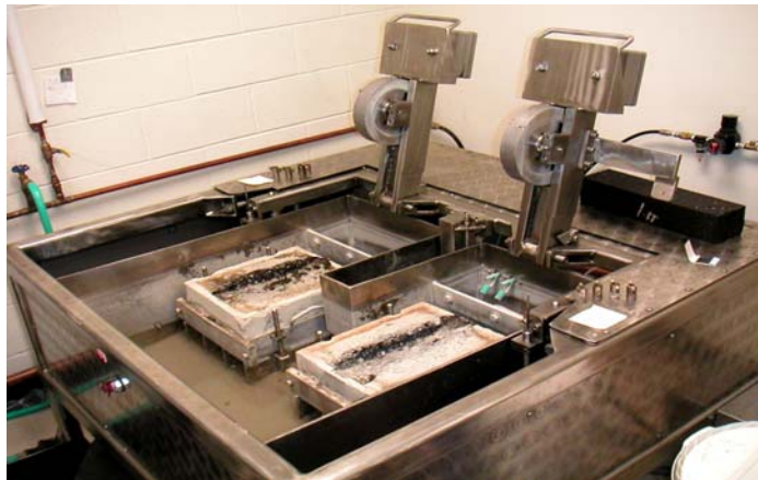
FIGURE 1. Hamburg Wheel Tester
