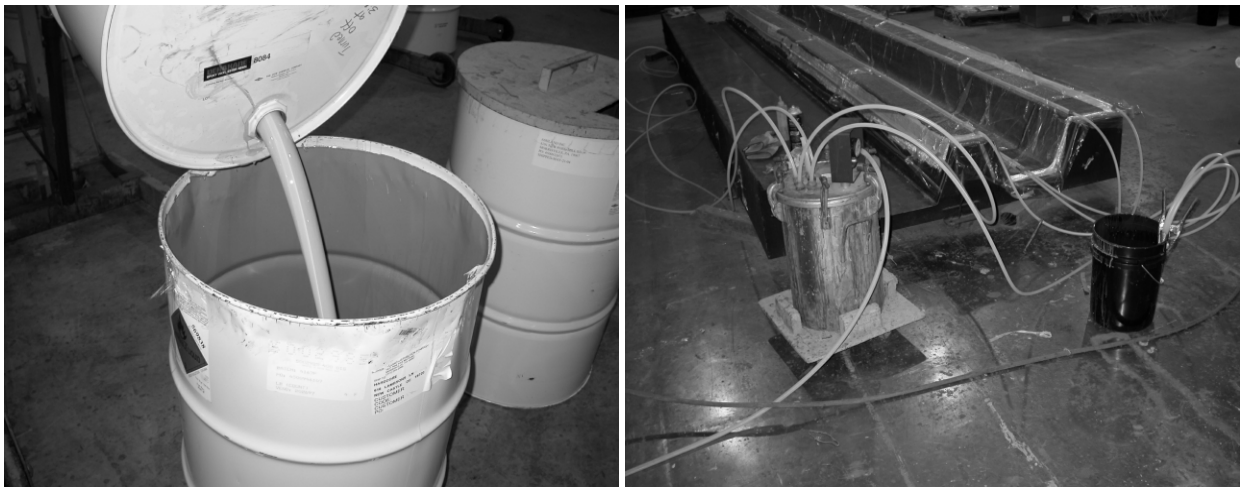
Figure 6. Example of VARTM process
