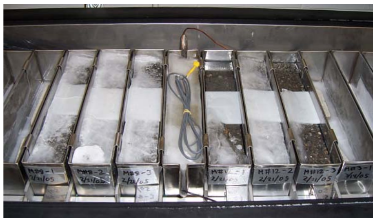
Figure 2. PCPC freeze-thaw test samples
