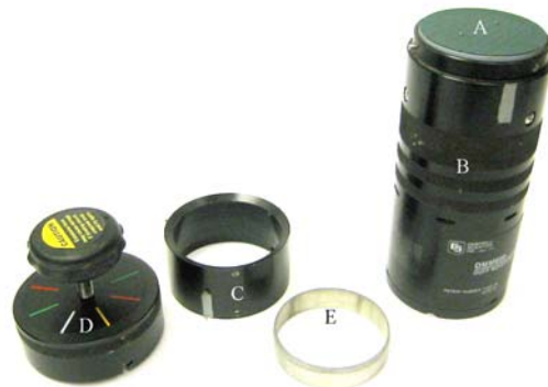
Figure 3. DMM600 components: (a) sensor plate/waveguides; (b) electronics housing; (c) sample chamber; (d) sample chamber cap, including compression knob (right) and compression plate; (e) special soil cutter tool (0.75 inches high by 2.88 inches in diameter)
