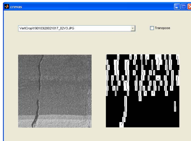
Figure 16. Strong crack, but noisy results
