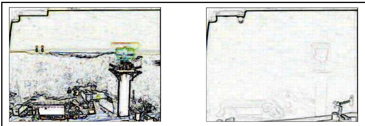
Figure 7. Edge-extracted images for the Hanscom AFB camera from a clear day (>40km visibility), left, and a low visibility day (< 100 m), right.
