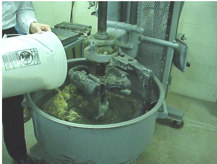
Figure 5. Mixing of UHPC
