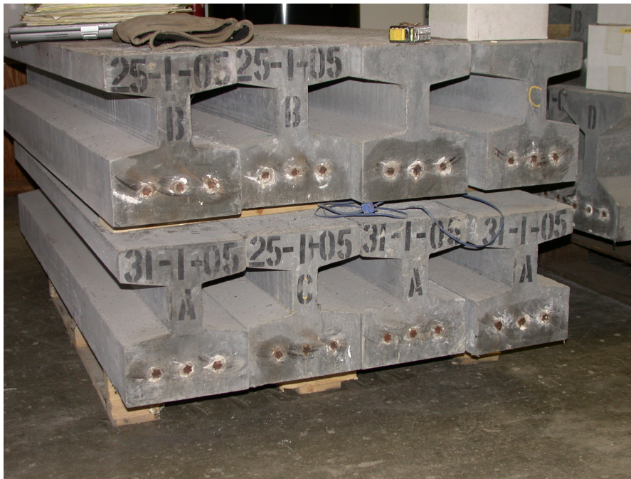
Figure 15. Ten-inch and 12-inch shear beams at Iowa State University
