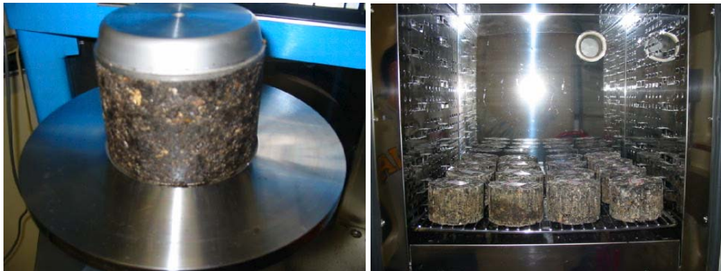
Figure 3. Gyratory compaction and curing process
