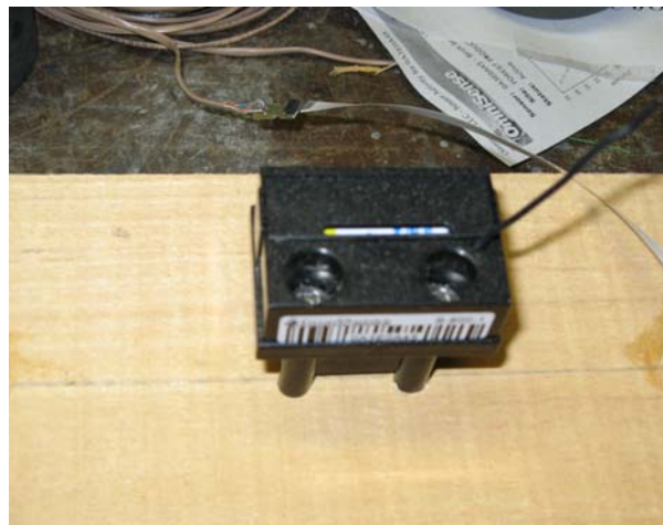
Figure 4. Omnisense wireless resistance pin sensor
