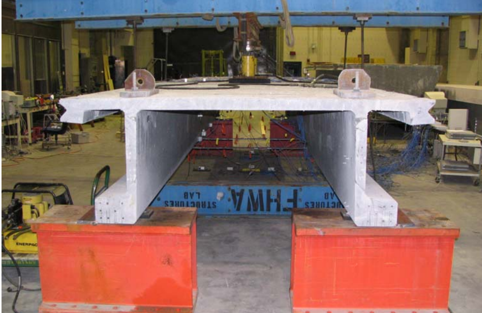
Figure 10. Transverse deck test
