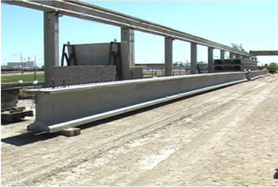
Figure 2. UHPC beams prior to shipping to bridge site
