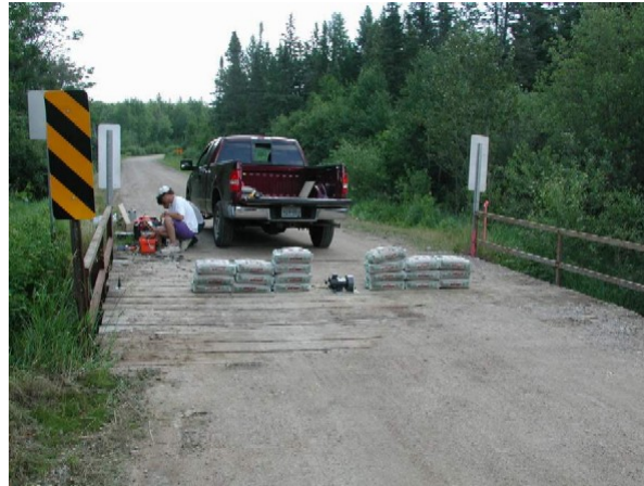
Figure 2. Measuring the response of a single-span timber bridge to forced vibration testing
