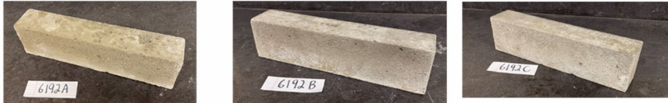
Mixture A after 300 F-T cycles
