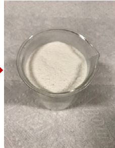
Powder blend with mineral powder coating: well-dispersed microspheres
