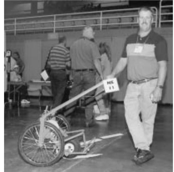
The Nebraska Department of Roads' (NDOR) Pavement Tape Dispenser, one of 13 NDOR innovations, places pavement markings during patching or armor-coating. The dispenser saves a lot of time and energy because no manual cutting or placement is involved.
