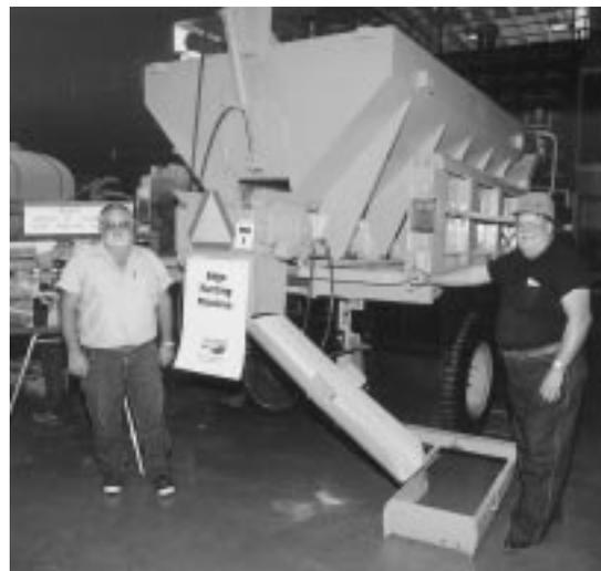
The Edge-Rutting Machine was designed and manufactured by the MoDOT Mendon maintenance crew to enable one person to fill edge ruts, low spots over culverts, and potholes. The machine has netted an increase in production of up to 600 percent in patching-related tasks since its invention in February 1998.
