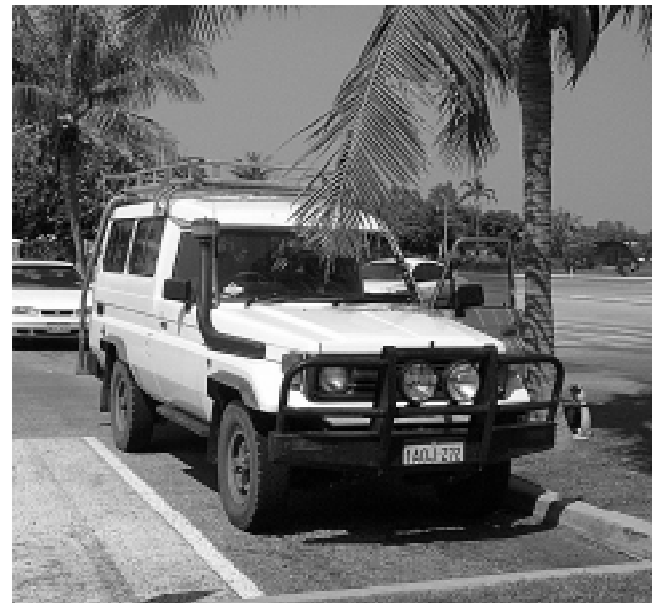
It's not uncommon in Australia to see four-wheel drive vehicles with bullbars (to protect the radiator and headlights from errant kangaroos) and snorkel (black air intake pipe going up the right windshield support with air cleaner on top, to get the air intake above the road dust). Photos here and bottom of page 3 courtesy of Chuck Jahren.
