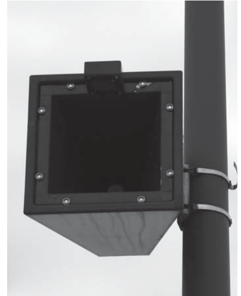
A wayside horn is a one-to-one replacement for a train horn. It is not required for a quiet zone.
