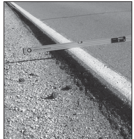
Figure 1. Edge drop-off was a feature of several granular shoulders examined in White's study
