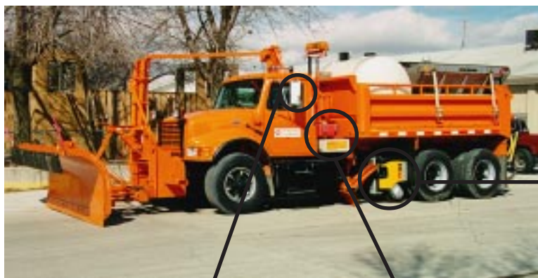
high-intensity warning lights Tri-State Signing New Hampton, Iowa
