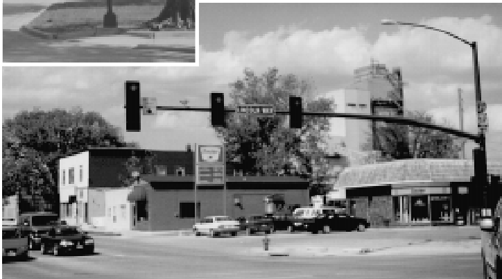
Replacing pedestal mounted signals (top photo) with mast arm mounted signals (bottom photo) contributed to a 36 percent crash reduction.
