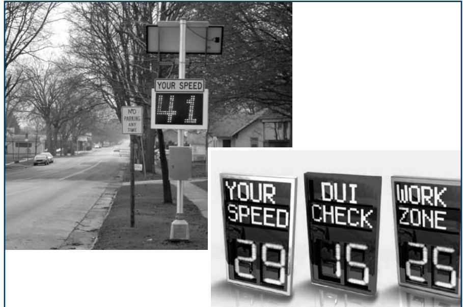
A speed display installed in Slater (left) and speed displays with variable messages (right). (All photos courtesy of Dr. Shauna Hallmark, InTrans, ISU)
