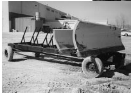
A storage rack assembled from scrap metal offers storage for wing plows. Photos courtesy of West Des Moines Public Works.
