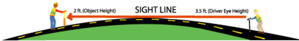
Figure 2. Sight rod (right) and target rod in use
