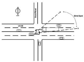
Obstructed vision at this intersection contributes to failure of eastbound traffic to yield right of way.
