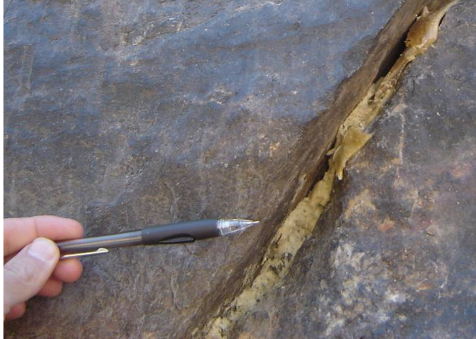
Figure 10. Photo. Cured PUR product infilling a discontinuity within rock mass.
