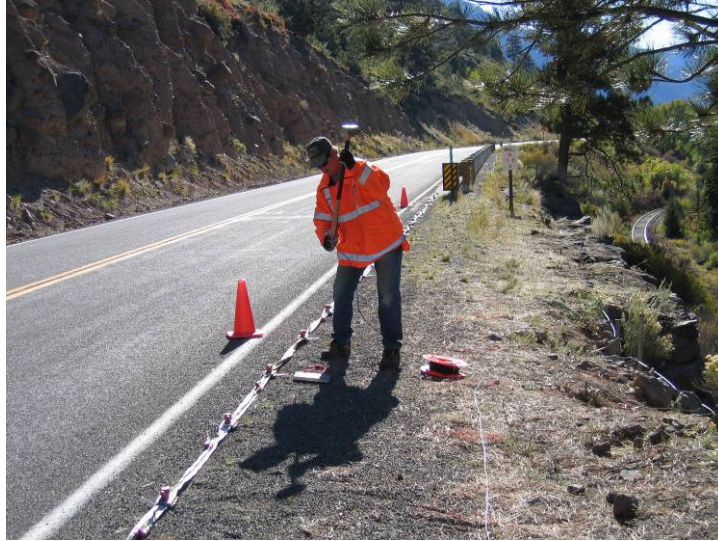
Figure 26. Photo. 2D seismic refraction line layout along roadway edge above retaining wall, including 24-channel “Landstreamer” geophone string and 20-lb triggered sledgehammer seismic source.
