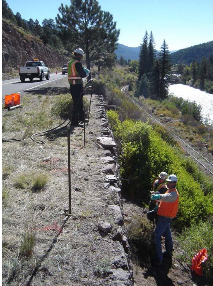
Figure 18. Photo. Jam-rods placed along the top of a well-built, well performing section of the study wall. No signs of wall settlement allowed placement of the injection rods closer to the wall face.
