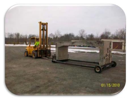
carrier is light enough to be moved around by one person guiding with the tongue, yet still strong enough to haul a 10-ton box culvert.
