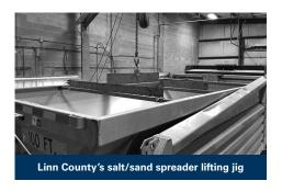
"For less than \$300 and a few hours of labor, Linn County has a safe, efficient and quick way to prep the sander for removal from the dump truck that also helps prevent injury," reads the entry. "The jig is made from steel, so we expect it will provide many years of service."
