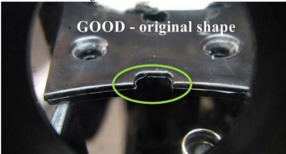
Figure 3: Groove with machine-manufactured dimensions.
