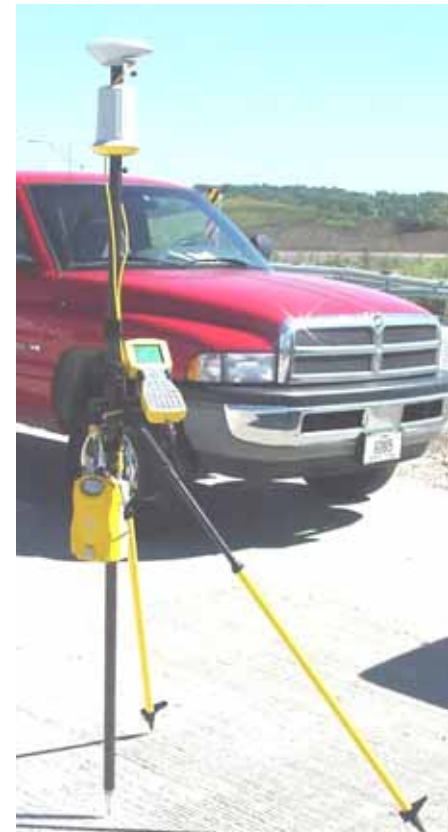
Typical GPS rover unit on roadway
