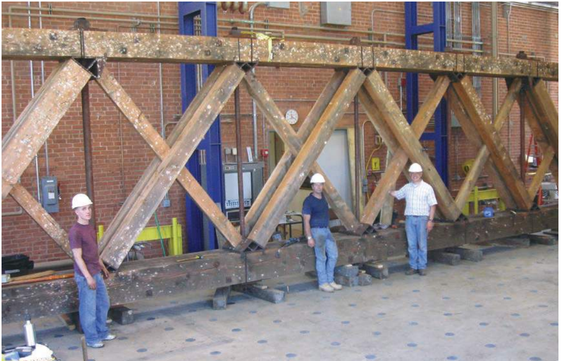
Figure 2.5 FHWA funded a joint project between HAER, Case Western Reserve University, and the National Society for the Preservation of Covered Bridges to study the Moose Brook Bridge (1918) in Gorham, New Hampshire, a Howe truss that was a victim of arson in 2004. The original castings were restored, and bridgeworker Tim Andrews reconstructed the salvaged trusses for testing in Case Western’s lab. Top 2.5a) The burned trusses sat idle for five years. HAER NH-48-3, Jet Lowe, photographer, 2009. Above 2.5b) The first truss assembled in the lab. Photograph courtesy Dario Gasparini, 2011.
