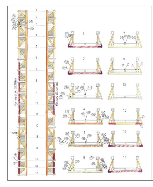
Color inventory map showing decay / deterioration in two different stages ( orange -> red) and intact parts (yellow). Mostly, red or purple is used when more than 30% of the cross section is damaged (depending on kind of damage).
