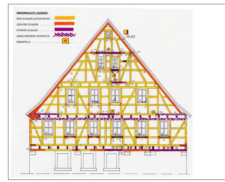
Simple map of a half timbered building. Inspection: one person one day. Costs: ~2'000 Euro (incl. travel). Savings ~50'000€. Most decay was internal / hidden / invisible and would have led to unplanned additional work and time (and cost) in conventional restoration.
