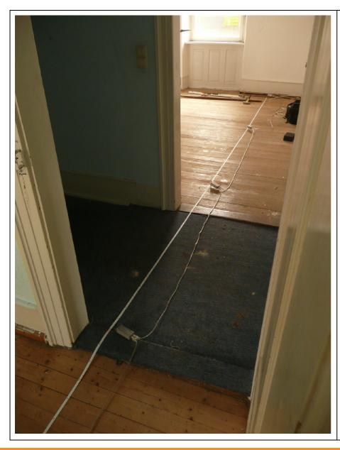
Determining length and potential connection of beams (on walls) across buildings without taking off the floor (or stucco) with the use of stress-wave sensors.
