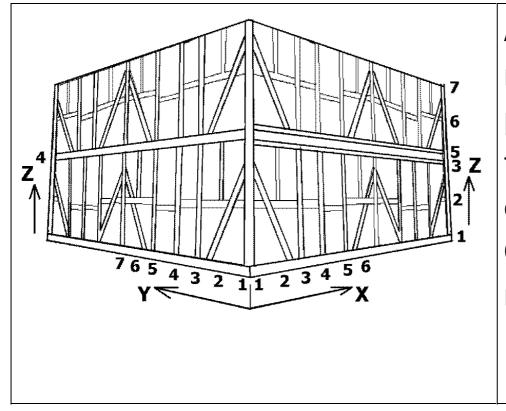
A simple coordinate system is prerequisite for clearly marking beams, parts, and connections and labeling them with a position (x,y,z) that cannot be mixed up later. Commonly, every structural axis is named with a number.
